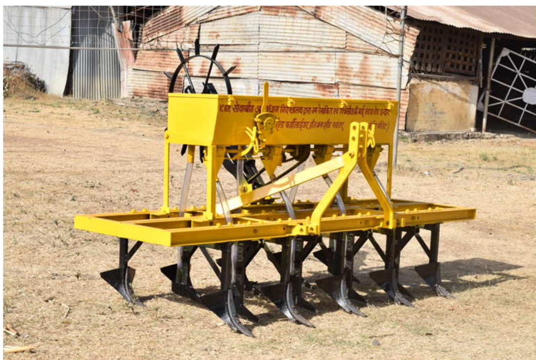
Fig. 7.1b : Ridge fertilizer drill cum seed planter (Inclined plate type)
