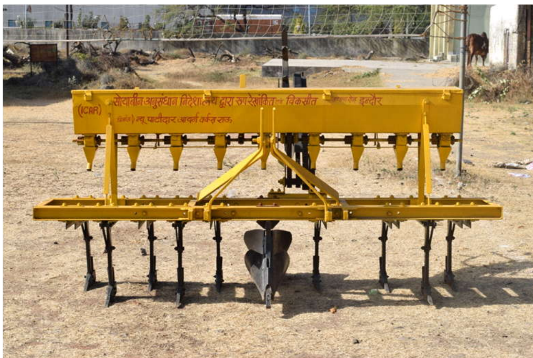
Fig. 7.1a : Single bottom BBF machine for Low HP tractors ( 30 HP to 40 HP )
