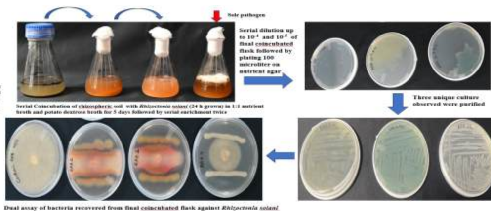
Fig. 3.2.3.4. Serial Coincubation Enrichment Technique (SCET): Rapid isolation of bacterial biocontrol agents
