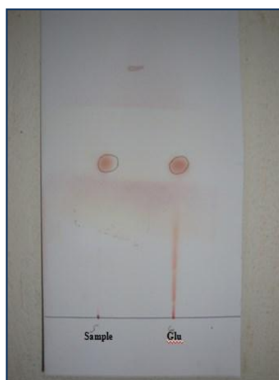
Plate 1: TLC plate showing the breakdown of PGA to glutamate
