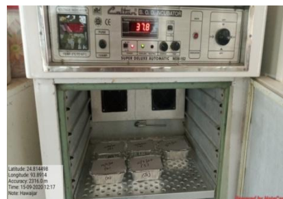
Cooked soybean kept in incubator for fermentation
